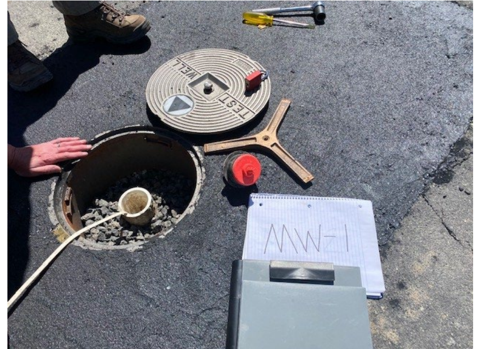
Measuring Static Water Level at MW-1S
